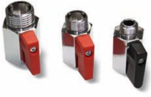
These small manual valves are suited for intercepting vacuum on vacuum cup holders and any small utility in which solenoid valves cannot be installed. They feature a hexagonal nickel-plated brass body, a chromed brass ball shutter and a seal in plastic material to guarantee a perfect seal. A lever on the ball shutter, rotated by 90°, allows opening or closing the valve with no effort.
